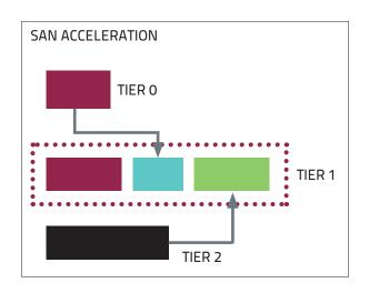
The other approach to leveraging solid-state storage is to use it as an extension of the disk controller cache to address peaks in storage performance demand. To accelerate reads and writes to disk drives, disk array storage controllers have always relayed on cache. However, a cache with volatile memory cannot be considered as a higher tier of storage and could be very limited in terms of scalability.
