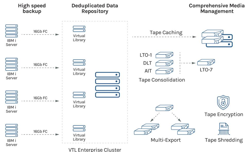
The virtual tape drives are presented to the IBM i servers via the front-end FC interfaces, and the back-end interfaces communicate with the deduplication repository to retain data on high-performance RAID 6 protected disk arrays for fast recovery and restore. The back-end interface can also attach to physical tape drives/libraries for export of VTL tapes for
