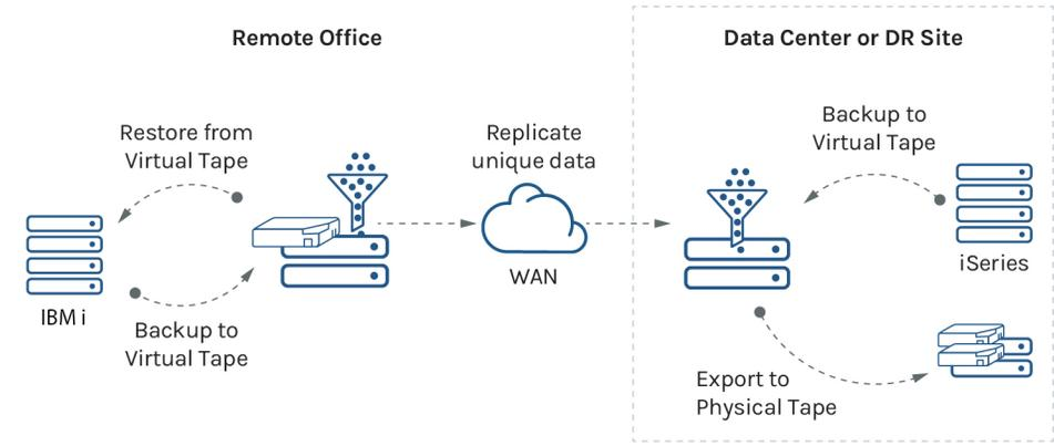
By using FalconStor VTL with IBM i, smaller offices and remote sites can electronically vault tapes across any distance using standard IP (WAN) networks, centralizing data at the DR site for long-term data protection, retention, and central tape creation. Data over the wire is encrypted (AES 256-bit) and data written from the FalconStor VTL directly to physical tape can also be encrypted (AES 256-bit), ensuring data is safe at all times.
