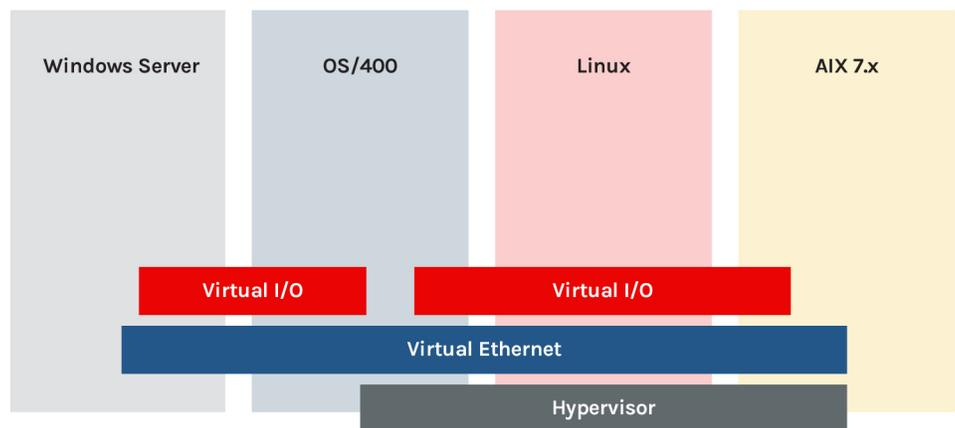
With LPAR, companies have both the power and flexibility to address multiple system requirements in a single machine to achieve server consolidation, business unit consolidation, a mix of production and test environments, and integrated clusters. LPARs are ideal for companies that want to run varied workloads in a single IBM i system. Licenses can be managed across partitions.
